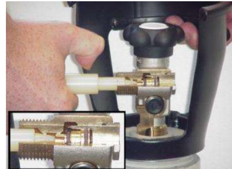
Tool used to check the functioning of RPV valves
